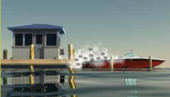
Blockage of boat exhaust by obstruction.
