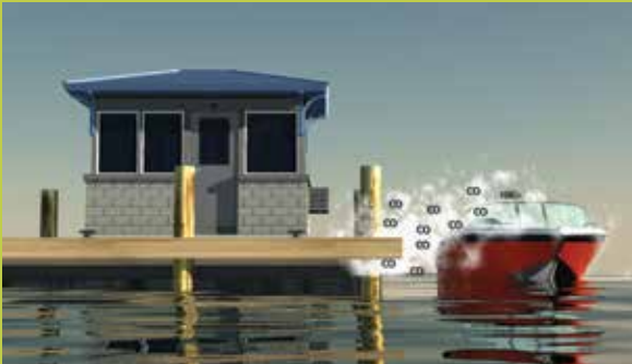
Exhaust traveling along obstruction.
