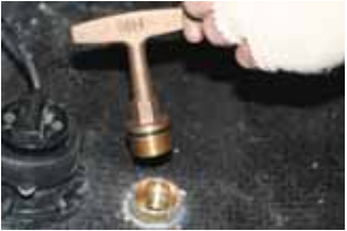
Figure 2-39. Bilge Drain Plug
