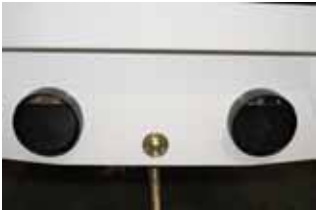
Figure 2-38. Transom Drain Plug
