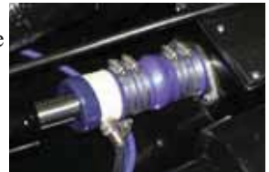
Figure 4-1. Drip Less Shaft Packing
