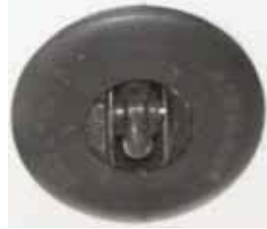
Figure 2-40. Thru-Hull Paddle Wheel Pickup
