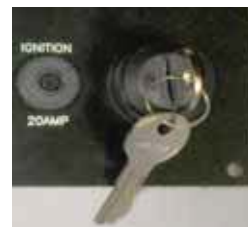
Figure 2-15. Remote Ignition Key Switch
