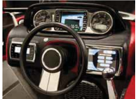
Figure 2-2. MaliView Dash with Malibu Touch Control (All Wakesetters)
