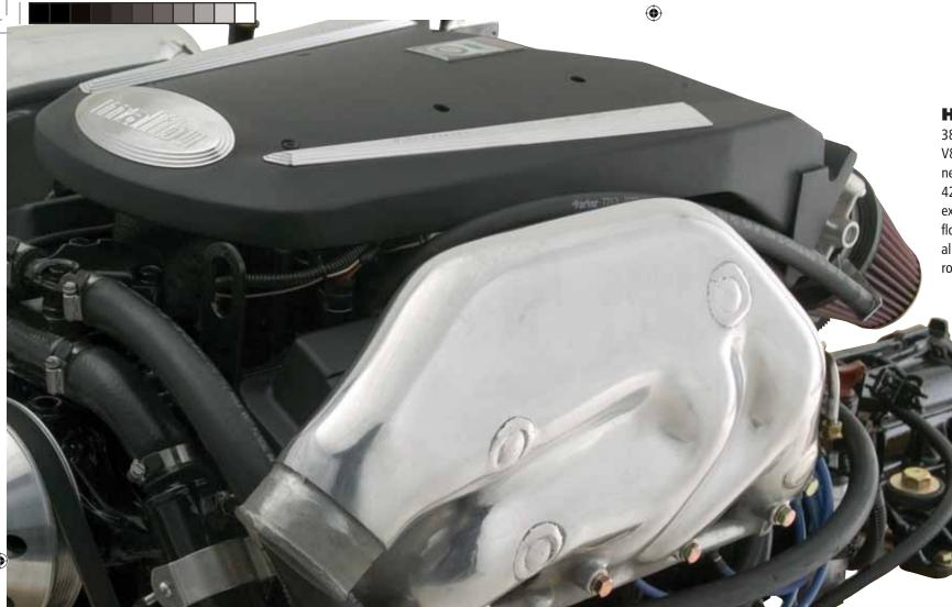
**Hammerhead 383.** The Hammerhead 383 (400 HP) is the most powerful 5.7L small-block V8 ever developed for inboard use. Its aggressive new appearance matches its 400 horsepower and 420 foot-pounds of torque. Capped with Malibu's exclusive intake plenum, it sports Indmar's highflow multi-port induction system, GM's FastBurn aluminum heads and Indmar-spec cam with 1.6:1 roller rockers for less friction, more power.
