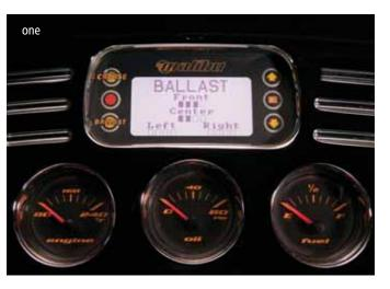
**one.** The Ballast Monitoring System data, which enables you to track and duplicate individual wake preferences, is now easily visible in the centered LCD graphical dash display, featuring a bar graph that shows ballast volumes in each tank.
