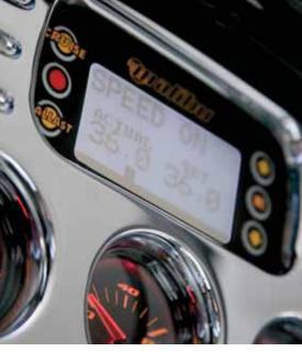
**Precision Pro Speed Control.** The new LCD graphical display in the center of the dash incorporates the industry's first standard world class cruise control for all water sports disciplines, from low speed surfing and boarding to crisp, steady slalom speeds.
