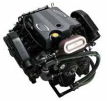
**Vortec 8100.** Vortec 8100 (425 HP) its 496 cubic-inch offers up to 450 horse power and 525 foot-pounds of torque. 9.1:1 high-compression Vortec heads turn out more usable power from every fuel charge. The MPFI aluminum intake manifold bolsters cylin-der-to-cylinder airflow distribution for cleaner, more dependable combustion. Finely tuned plenum runners and the coil-near-plug ignition system (distributorless) enhance low-end torque and delivers awesome power.
