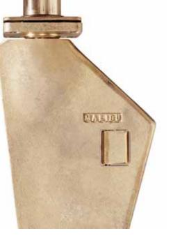
Adjustable Rudder. Customize the torque of the rudder for the perfect pull or driving preference with the twist of an allen screw on Malibu's exclusive adjustable rudder. Malibu puts the controls in your hands.
