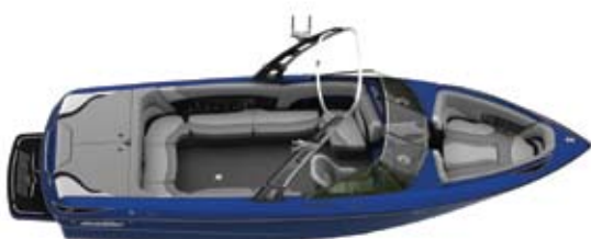
Length 24' 7"/7.50m Beam 102"/2.59m Draft 27"/0.69m Capacity 16 persons Fuel 87 gal./329L Weight 3900lbs./1769k
