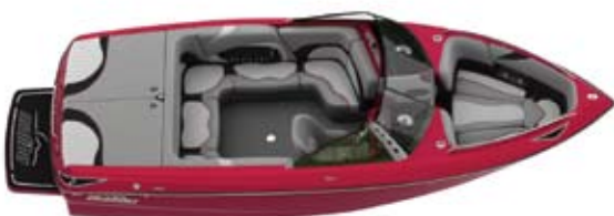
Length 20'/6.10m Beam 98"/2.49m Draft 22"/0.56m Capacity 11 persons Fuel 46 gal./174L Weight 3200lbs./1451k
