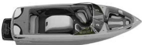
Length 20' 6" / 6.25m Beam 93.5" / 2.37m Draft 22" / 0.56m Capacity 9 persons Fuel 41 gal. / 155L Weight 2600lbs. / 1179k
