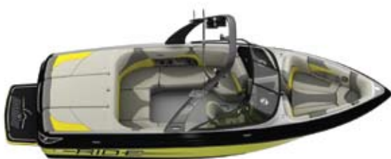
Length 21' 6"/6.55m Beam 100"/2.54m Draft 24"/0.61m Capacity 11 persons Fuel 46 gal./174L Weight 3500lbs./1587k
