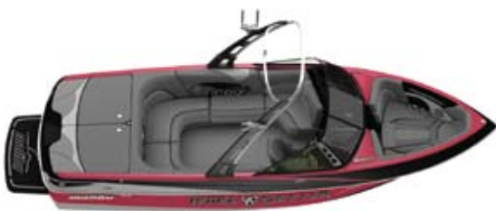
Length 21' 6"/6.55m Beam 100"/2.54m Draft 24"/0.61m Capacity 11 persons Fuel 46 gal./174L Weight 3500lbs./1587k
