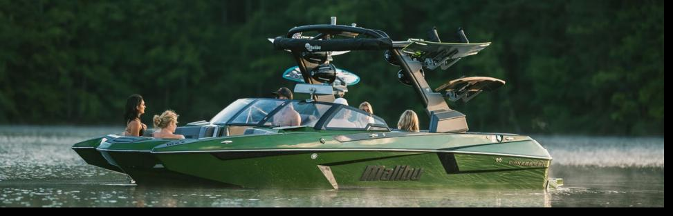
23 MXZ 23' | 16 Capacity | Max Ballast: 4.670lbs | Hull Type: Wake Plus | Torque: 400-606ft-lbs | Weight: 5,400lbs
