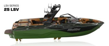
LENGTH: 25' CAPACITY: 18 People HULL TYPE: Wake Plus FUEL: 103 gal TORQUE: 460-606ft-lbs WEIGHT: 6,175 LBS MAX BALLAST: 5,180 lbs.\*
