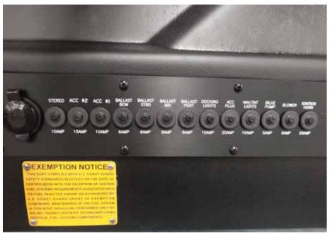
Figure 2-2. Circuit Breaker Panels
