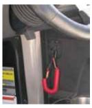
Figure 2-6. Emergency Engine Stop Switch
