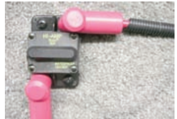
Figure 4-12. Main Circuit Breaker
