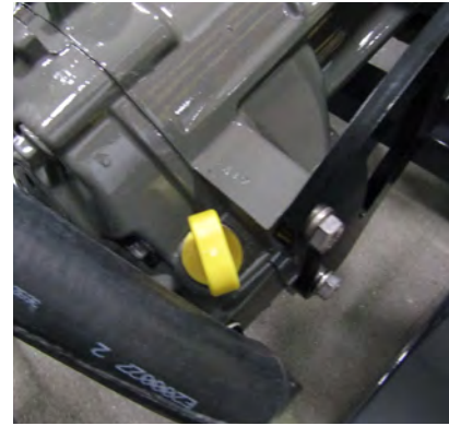
Transmission dipstick (red); V-Drive dipstick (yellow).
