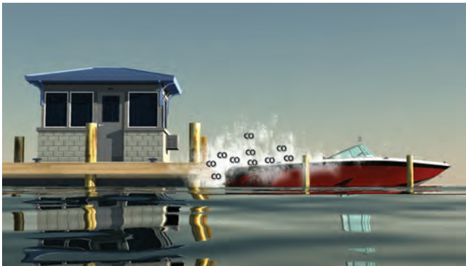
Blockage of boat exhaust by obstruction.
