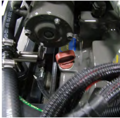
Transmission dipstick (red); V-Drive dipstick (yellow).
