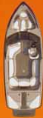
SUNSCAPE 23 LSV Length 23'7"/7.01m Beam 102"/2.59m Draft 27"/0.69m Capacity 14 persons Fuel 55 gal./208L
