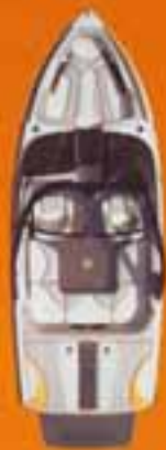
SUNSCAPE 21 LSV Length 21'6"/6.51m Beam 88"/2.49m Draft 24"/0.61m Capacity 12 persons Fuel 46 gal./174L
