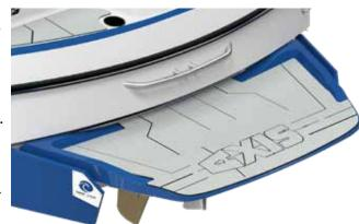
hull and deck finishes The majority of the finish surface of the hull and deck is a fiberglass-reinforced resin. While the boat material is sturdy, to ensure an enjoyable experience while boating, the fiberglass-andresin layers and gel coat finish (where the paint is embedded) is very thin—only a few millimeters in depth. To keep it looking like new, it is important to keep it clean and waxed.
