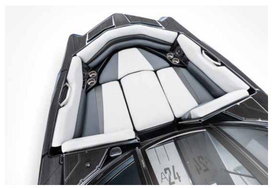
Armrests are intended to be used only as armrests. Any excessive weight placed on an armrest, even briefly, can result in failure of the armrest. This is not covered under warranty, and could also result in injury. In moving armrests up and down, use caution to avoid pinching fingers or skin.
