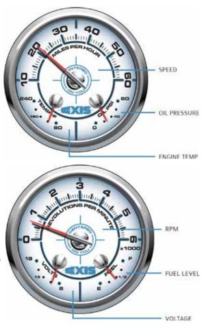
during engine operation is above 13.5 volts. See the battery information that follows in this section of the Owner's Manual for additional details regarding the proper charging and battery switch designation.
