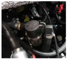
Raw water from the lake/river/sea is drawn into the boat to cool the engine and drive train. Even in closed cooling systems, it is necessary to circulate water in part of the system. To protect the system, an optional sea strainer may be installed near the raw water intake and serves the purpose of keeping debris from entering the cooling system and causing eventual engine failure. As with any kind of strainer, it is necessary to regularly clean it so that water can flow unimpeded.
