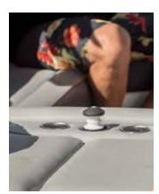
All models are equipped with at least one ski pylon. The tower has a pylon mount that can be used for wakeboarding and some other water activities. Generally, the pylon is located between the lounge lean-back seats and the sun deck area.
