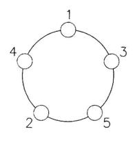
Follow these instructions for ensuring proper installation and torque for the lug nuts:
