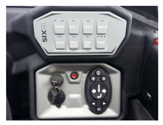
**Heater:** Press this button once to turn the Heater ON with the blowers operating on HIGH. The LED on the left side of the button will light. Press the button a second time to reduce the blowers to LOW. The LED on the right side of the button will light. Press a third time to turn the Heater OFF.
