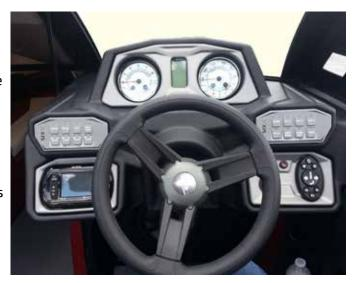
The Axis instrument panel features two (2) five-inch (5") gauges, which provide real-time information about important drive train functions.
