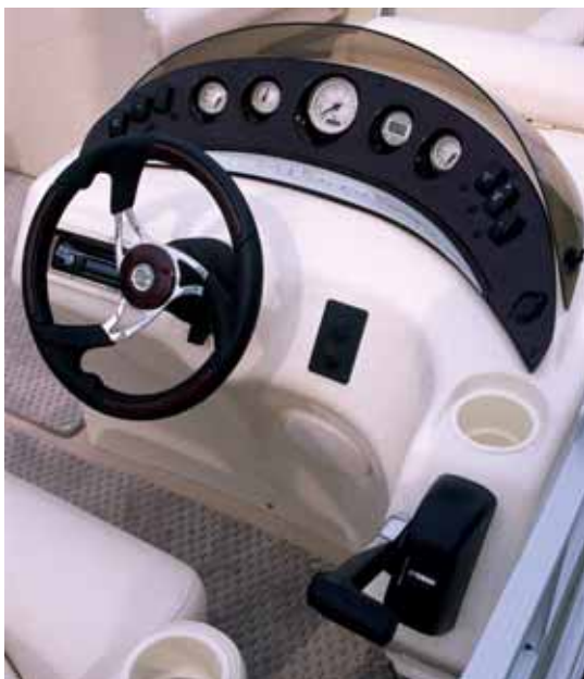
▲ G Series Console One-piece fiberglass unit with handsome wood grain dash insert and chrome ringed, fog resistant gauges. *Shown with optional deluxe steering wheel
