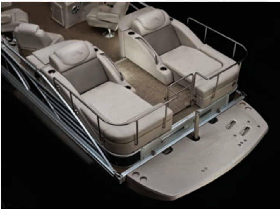
Stern lounge seating Seagrass aft flooring Removable stainless steel ski pylon Swim platform with telescoping boarding ladder
